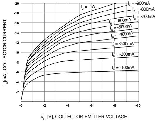
Figure 1. Static Characteristic
