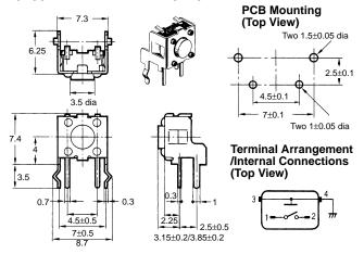
Vertical, Projected Plunger Type (Height: 6.15 mm)
