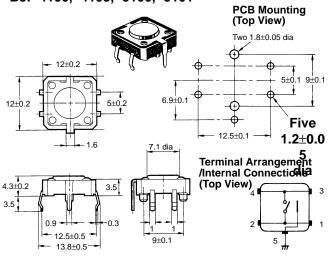
Standard, Long Life Expectancy, High Reliability, Projected Plunger Type (without Ground Terminal) B3F-4050, -4055, -5050, -5051 Standard, Long Life Expectancy, High Reliability, Projected Plunger Type (with Ground Terminal) B3F-4150, -4155, -5150, -5151
