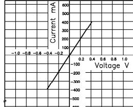
**Fig.9** Off state leakage current
