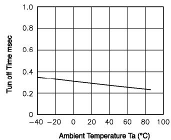
**Fig.5** LED operate vs. ambient temperature
