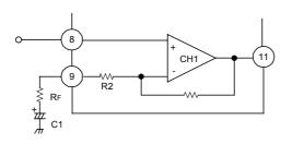
i) Fixed voltage gain (Pin 9 connected to GND directly)
