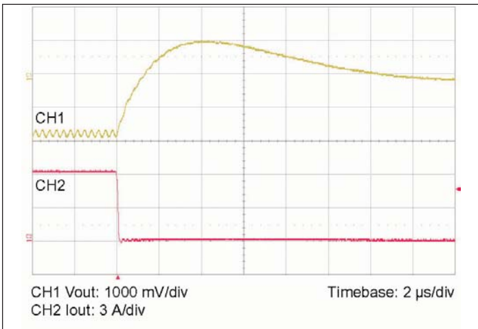
Figure 11— 6.3-0 A load step with 47 \mu F input capacitance.
