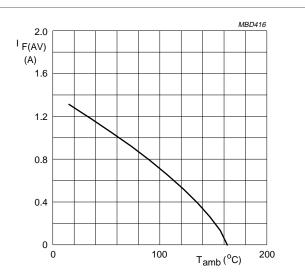
$\label{eq:rescaled} \begin{aligned} &a=1.42; \ V_R=V_{RRMmax}; \ \delta=0.5. \\ & \text{Device mounted as shown in Fig.8.} \\ & \text{Switched mode application.} \end{aligned}$
