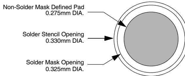
Figure 5. Recommended Non-Solder Mask Defined Pad Illustration
