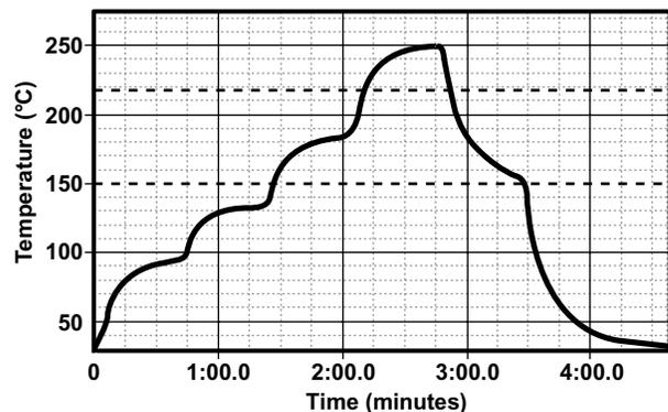
Figure 7. Lead-free (SnAgCu) Solder Ball Reflow Profile
