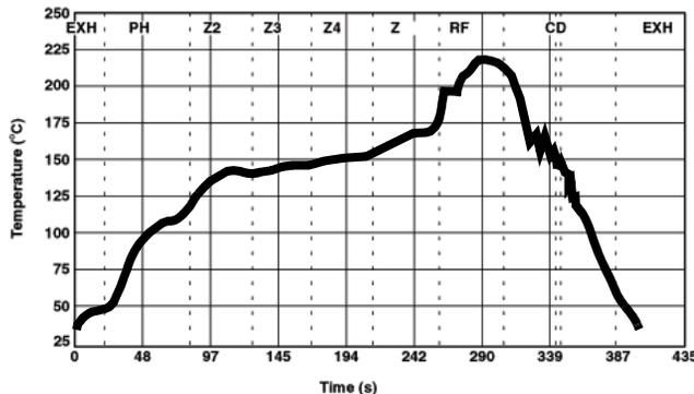
Figure 6. Eutectic (SnPb) Solder Ball Reflow Profile
