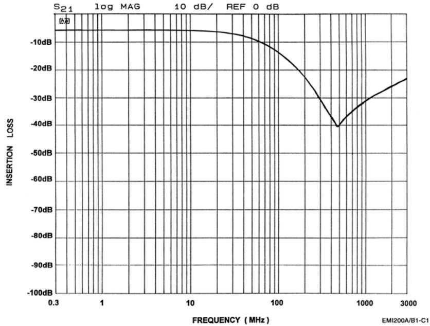
**Figure 1. Microphone 1 Circuit (B1-C1) EMI Filter Performance**
