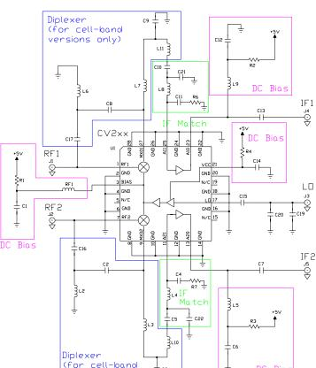
Printed Circuit Board Material: .014" FR-4, 4 layers, .062" total thickness
