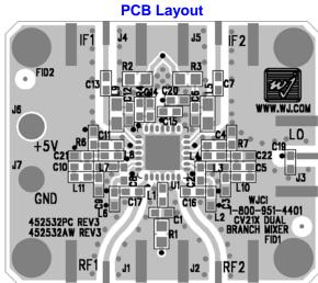
Circuit Board Material: .014" FR-4, 4 layers, .062" total thickness
