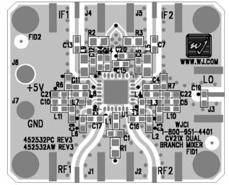
CV221-2A: The application circuit can be broken up into three main functions as denoted in the colored dotted areas above: RF/IF diplexing (blue), IF amplifier matching (green), and dc biasing (purple). There are various placeholders for chip components in the circuit schematic so that a common PCB can be used for all WJ dual-branch converters.
