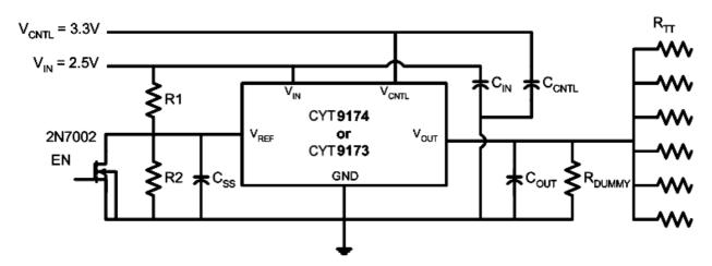
$R_1 = R_2 = 100K\Omega$ ,  $R_{TT} = 50\Omega/33\Omega/25\Omega$
