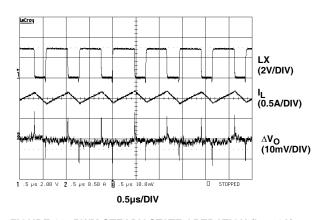
FIGURE 16. PWM STEADY-STATE OPERATION ( $I_O = 1A$ )
