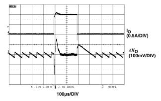
FIGURE 19. LOAD TRANSIENT RESPONSE (22mA to 1A)
