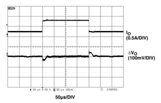
FIGURE 21. PWM LOAD TRANSIENT RESPONSE (0.25A TO 0.75A)
