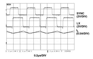
FIGURE 17. EXTERNAL SYNCHRONIZATION TO 2MHz
