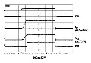
FIGURE 14. ENABLE AND SHUT-DOWN
