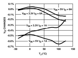
FIGURE 7. PWM MODE LOAD/LINE REGULATIONS vs JUNCTION TEMPERATURE
