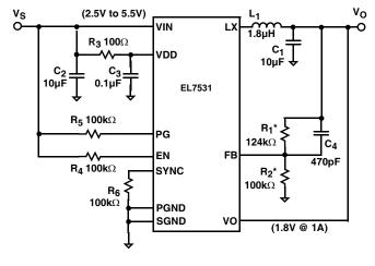
$V_0 = 0.8V (1 + R_1 / R_2)$
