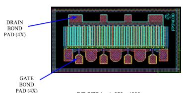
DIE SIZE ( $\mu m$ ): 650 x 1300 DIE THICKNESS: 100  $\mu m$  BONDING PADS ( $\mu m$ ): >70 x 65
