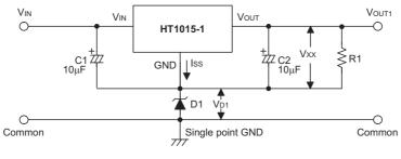
$V_{OUT1} = V_{XX} + V_{D1}$
