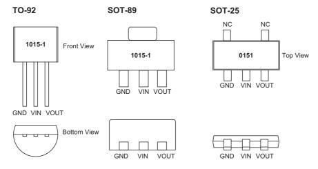
Note: For lead free devices, TO-92 package will add a "#" mark at the end of the date code, whereas SOT-89 and SOT-25 packages will add a "#" mark at the end of the marking.
