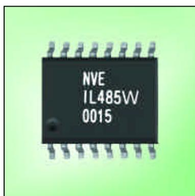
The IL485W is a galvanically isolated, high-speed differential bus transceiver, designed for bi-directional data communication on balanced transmission lines. The IL485W uses patented IsoLoop® technology and is the first isolated RS-485 interface available in a standard 16 pin SOIC package, which meets the ANSI Standards EIA/TIA-422-B and RS485.
