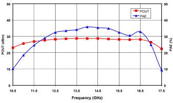
Figure 1. Output Power and Power Added Efficiency vs. Frequency at  $V_{\text{DD}}$  = 8V and  $P_{\text{in}}$  = 12 dBm.
