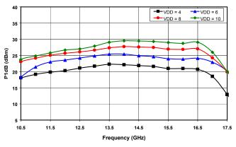
Figure 3. 1dB Compression Point vs. Drain Voltage
