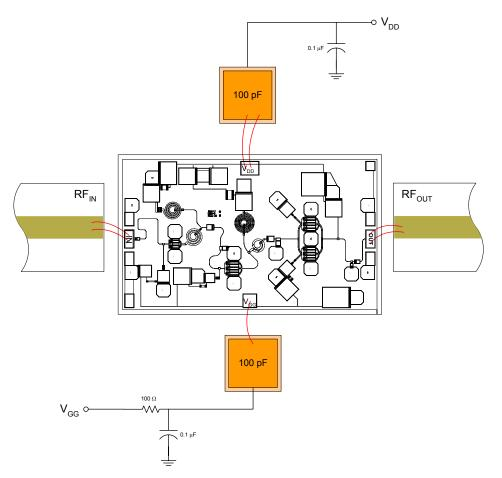
Figure 6. Recommended operational configuration. Wire bond as shown.
