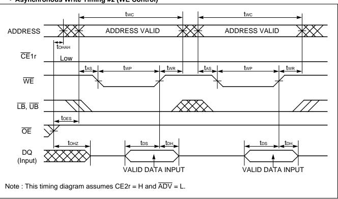
• Asynchronous Write Timing #2 (WE Control)
