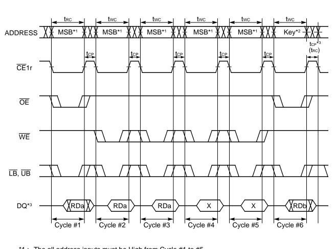
• Configuration Register Set Timing #1 (Asynchronous Operation)
