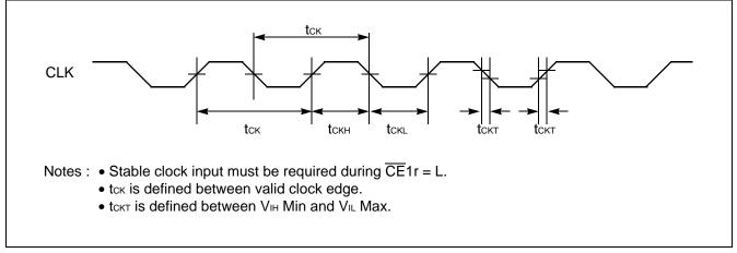
• Address Latch Timing (Synchronous Mode)
