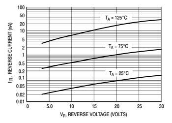
Figure 5. Reverse Current versus Reverse Voltage
