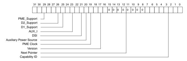
bit 31-27 : PME\_Support, read only indicates the power states in which the function may assert LANWAKE pin.
