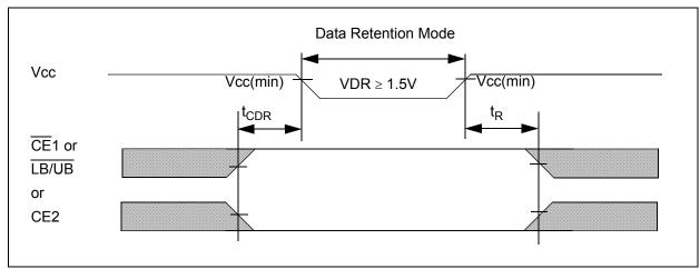
Note: Full device operation requires linear Vcc ramp from VDR to Vcc(min) > 100  $\mu s$
