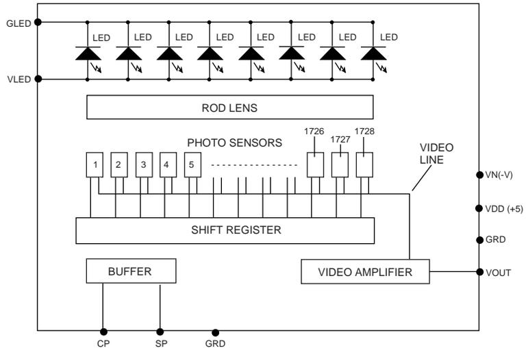
Figure 2. PI240MC-A4 Module Block Diagram
