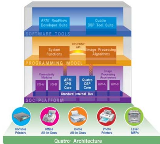
By pairing the ARM CPU core with the Quatro DSP core, the Quatro solution provides OEMs with a unique combination of high performance processing and easy-to-use programmability. The ARM CPU core, the established leader in embedded CPU cores, delivers high performance system and control processing with dense code size and a highly regarded software development tool suite.
