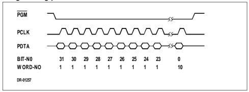
The  $\overrightarrow{PGM}$  pin is pulled low and the PCLK pin should be clocked with an external clock. The programming data on the PDTA pin must be stable during the rising edge of the clock signal on PCLK.
