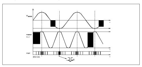
The output on pin FOUT is a pulse density signal representing the instantaneous power/ energy measurement. The minimum timing characteristics are shown in the following diagram.
