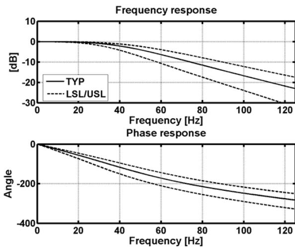
**Figure 3** Frequency response of SCA3000-D01 in measurement mode
