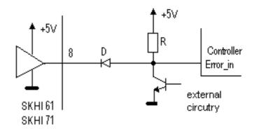
Fig. 2 ERR-Signal in an "open-collector"-circuit
