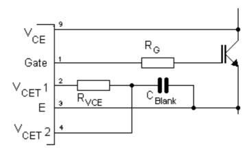
Fig. 4 Connection principle of a power switch with a specifically adjusted V<sub>CE</sub>-threshold
