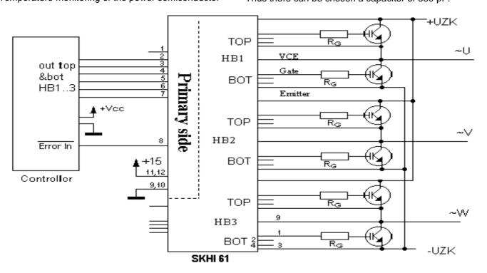
Fig. 7 SKHI 61 block diagram
