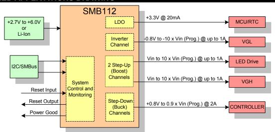
Figure 1: Applications schematic featuring the SMB112 Five-channel, programmable DC-DC controller Note: This is an applications example only. Some pins, components and values are not shown.
