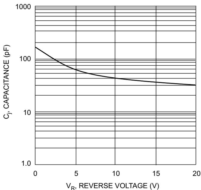
Fig. 3 Typ. Junction Capacitance vs Reverse Voltage
