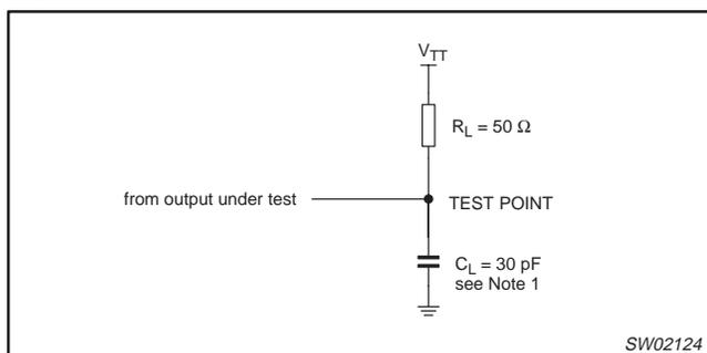
Figure 1. Load circuitry
