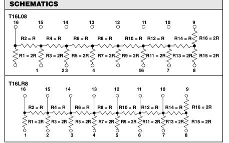
$R1/R2 = 2 \pm 1 \%.$   $R1/R3 = 1 \pm 1 \%.$   $R1/R4 = 2 \pm 1 \%.$   $R1/R5 = 1 \pm 1 \%.$   $R1/R6 = 2 \pm 1 \%.$   $R1/R7 = 1 \pm 1 \%.$   $R1/R7 = 1 \pm 1 \%.$   $R1/R8 = 2 \pm 1 \%.$   $R9/R10 = 2 \pm 0.5 \%.$   $R11/R12 = 2 \pm 0.4 \%.$   $R15/R13 = 1 \pm 0.2 \%.$   $R15/R14 = 2 \pm 0.2 \%.$
