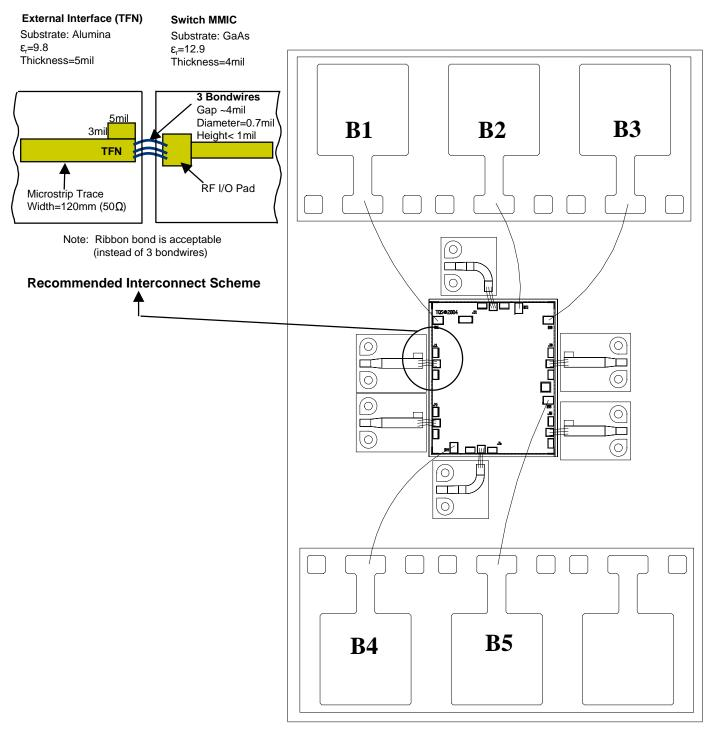
Note: Unused Ports should be terminated with 50  $\Omega$ .
