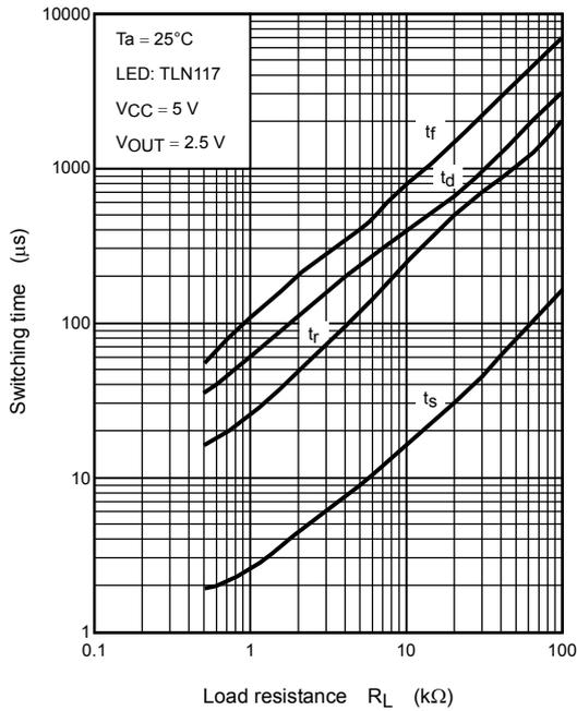
Switching characteristics (saturation) (typ.)
