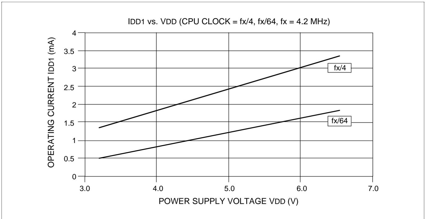
Figure 47. V<sub>DD</sub> VS. I<sub>DD1</sub>
