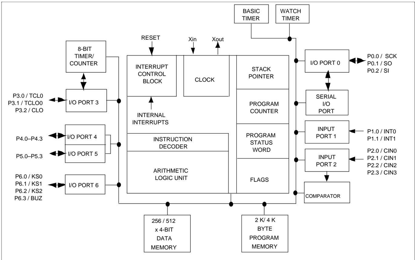
Figure 1. KS57C0002/0004 Block Diagram
