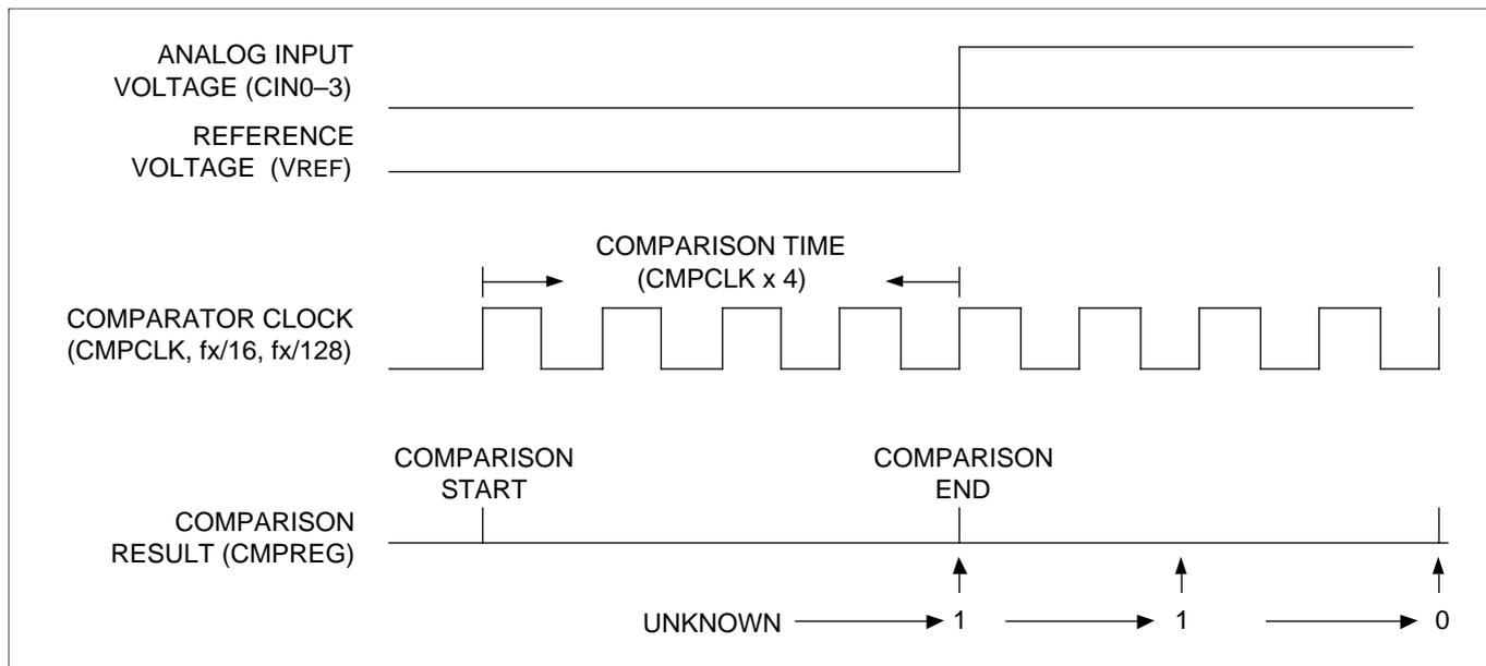
Figure 32. Conversion Characteristics
