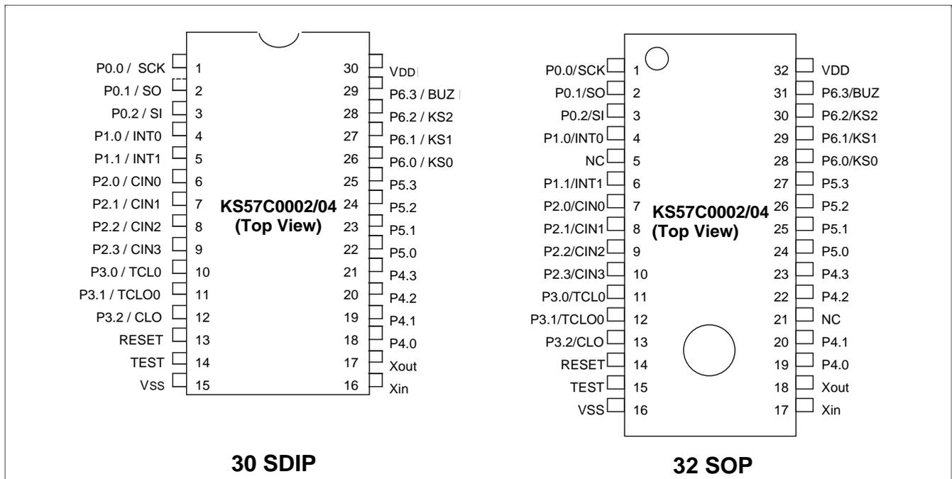
Figure 2. KS57C0002/0004 Pin Assignments (32 SOP, 30 SDIP)
