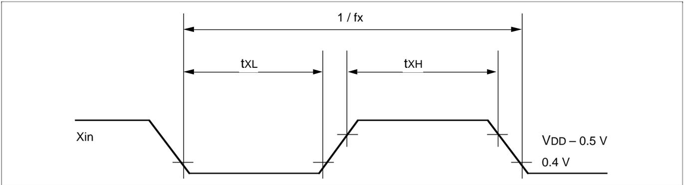
Figure 40 Clock Timing Measurement at  $X_{in}$
