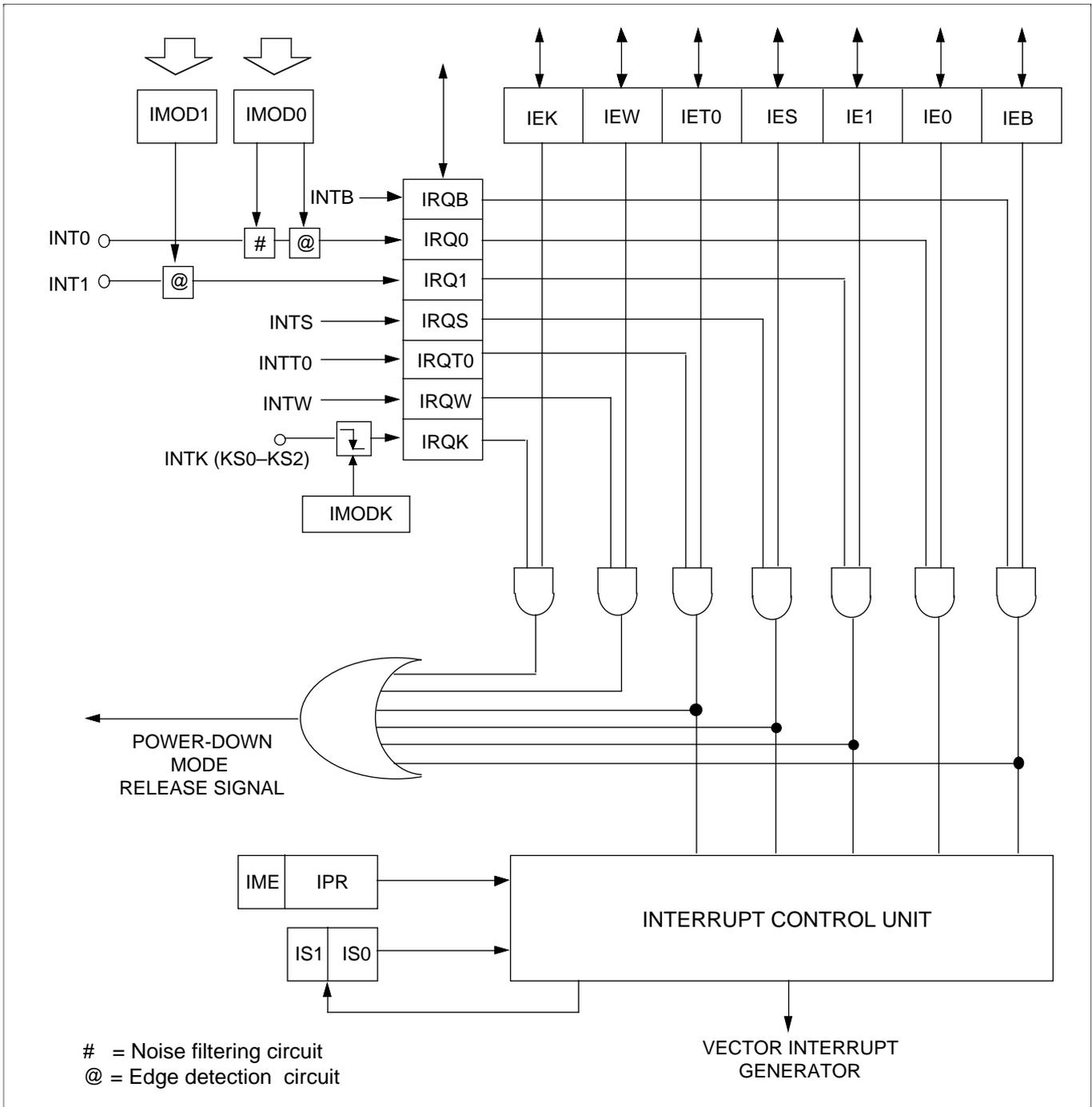
**Figure 15. Interrupt Control Circuit Diagram**
