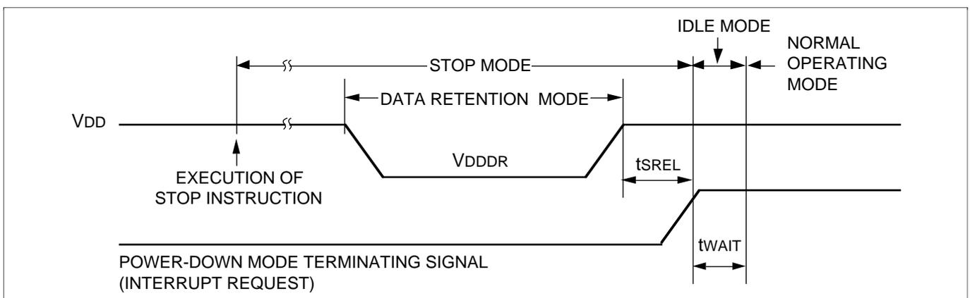
**Figure 39. Stop Mode Release Timing When Initiated By Interrupt Request**
