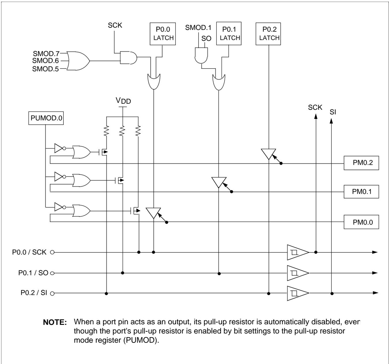
Figure 21. I/O Port 0 Circuit Diagram
