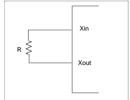
Figure 19. RC Oscillator (only for the KS57C0002)
