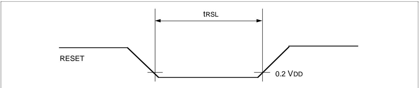
Figure 42. Input Timing for  $RESET$  Signal
