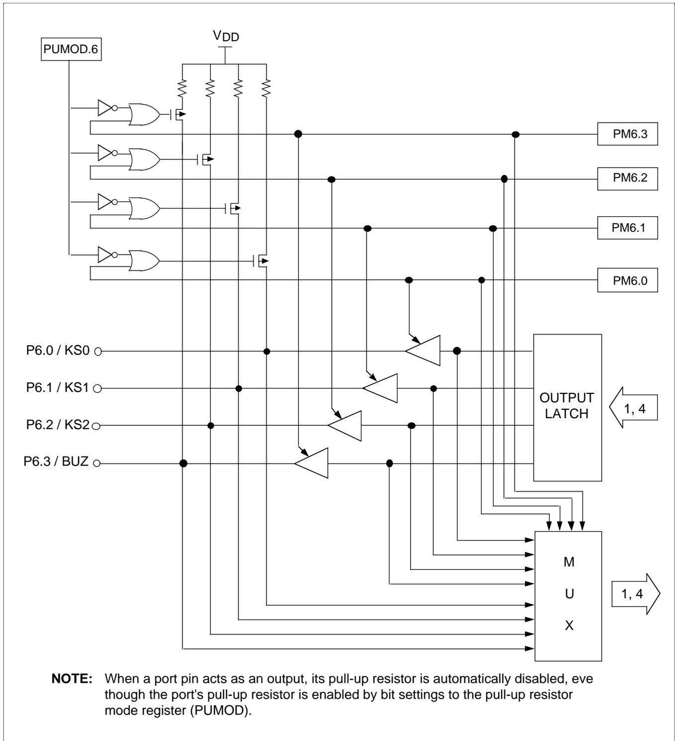
Figure 26. Port 6 Circuit Diagram
