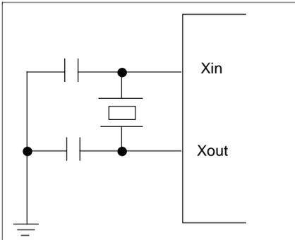
Figure 17. Crystal/Ceramic Oscillator
