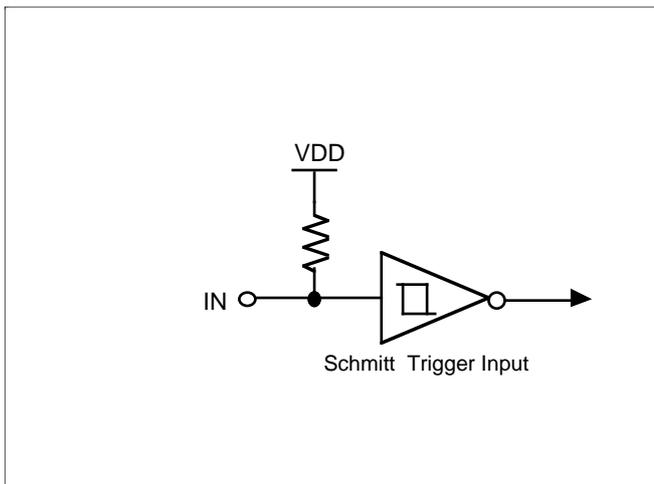
Figure 11. Pin Circuit Type 9
