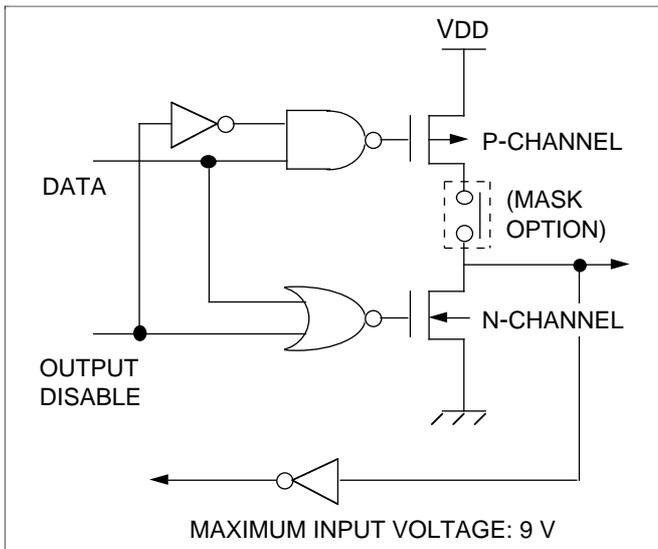
Figure 9. Pin Circuit Type 7
