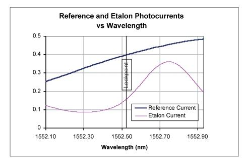
In order to lock the LMC10NEJ wavelength, a control circuit should be used which maintains the laser submount temperature constant over life and then controls the wavelength by varying the laser forward current to keep the ratio of the etalon and reference photodiode currents (Locking Ratio) constant. This may be achieved by keeping the discrimination value (LR x  $I_{ref}$ ) –  $I_{et}$ ) at zero, where LR is the target Locking Ratio.
