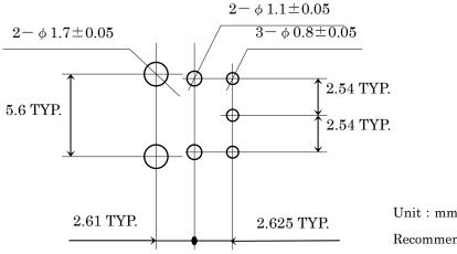
Recommended PCB thickness : 1.6mm
