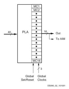
Figure 2: CoolRunner-II CPLD Function Block
