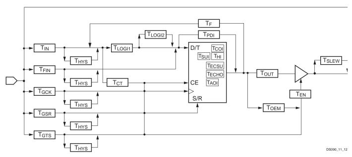
Figure 11: CoolRunner-II CPLD Timing Model
