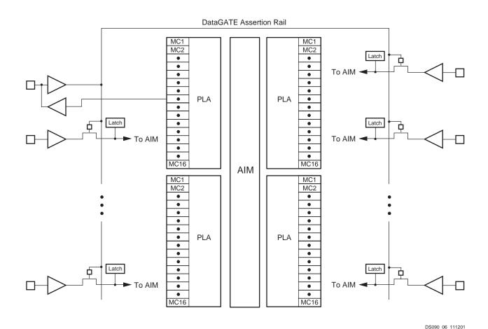
Figure 6: DataGATE Architecture (output drivers not shown)
