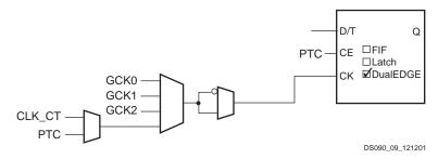
Figure 9: Macrocell Clock Chain with DualEDGE Option Shown
