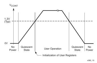
Figure 12: Device Behavior During Power Up
