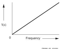
Figure 5: CMOS  $I_{CC}$  vs. Switching Frequency Curve
