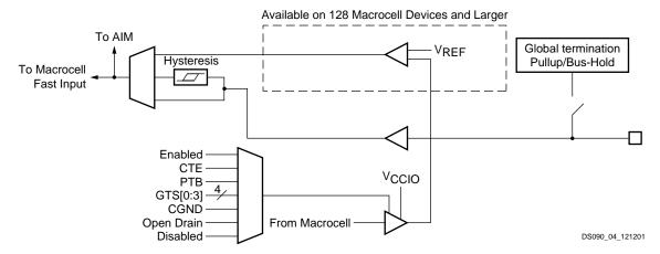
Figure 4: CoolRunner-II CPLD I/O Block Diagram
