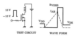
$$\begin{split} R_G &= 25~\Omega \\ V_{DD} &= 25~V,~L = 368~\mu H \end{split}$$
