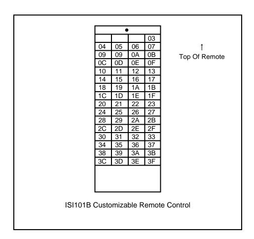
Illustration shows key locations of matching ISI101 "Customizable Standard" Remote Control and codes produced for each key location.
