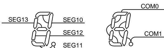
Figure 15-6 Example of COM, SEG Pin Connection
