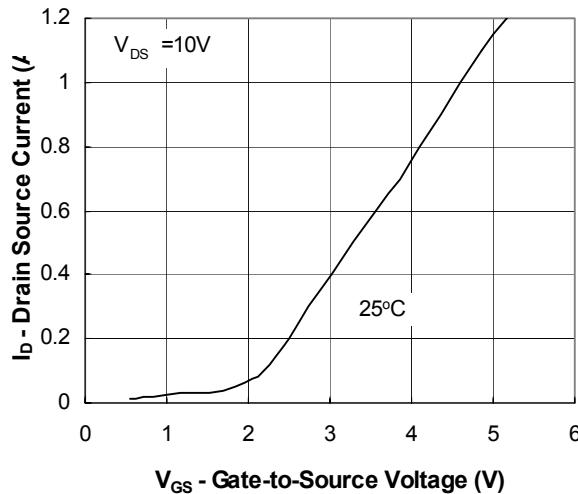
Fig. 2. Transfer Characteristics
