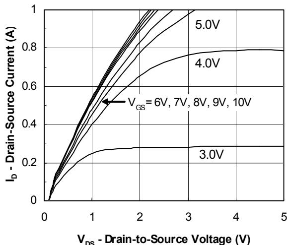
Fig. 1. Output Characteristics
