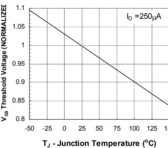
Fig. 5. Threshold Voltage vs. Temperature
