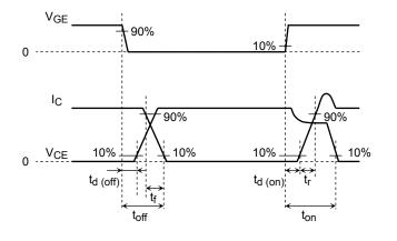
Note2: Switching loss measurement waveforms
