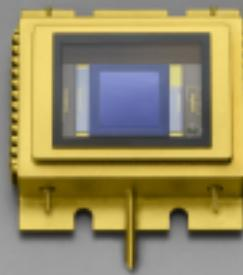
S8665-0909 is an FFT-CCD area image sensor featuring low noise and low dark current (MPP mode operation). The output charge can be integrated for long periods of time even at low light levels, allowing a wide dynamic range.
