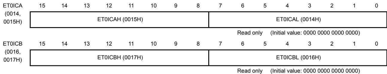
Note: Since capturing is restored by reading the upper byte of the capture register A, read capture register B before reading capture register A. Read capture register A from lower byte to upper byte.
