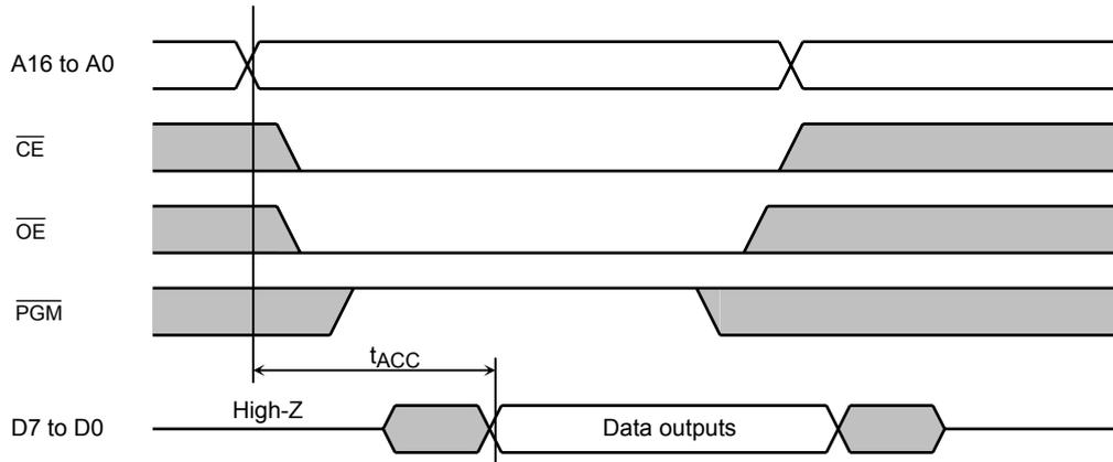
(2) High-speed programming operation (T<sub>opr</sub> = 25 ± 5°C, V<sub>DD</sub> = 6.25 ± 0.25 V)
