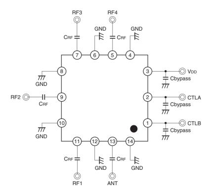
When using this IC, the following external components should be used:
