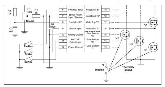
Another possibility is the use of a *Hall effect switch*. When the current through the driver MOSFETs reaches a certain threshold, the magnetic field induced in the sense coil will exceed the Hall effect switch threshold. The Hall effect switch should then switch to the "ON" state, and in that way pull the Disable input low. This in turn switches off all drivers.
