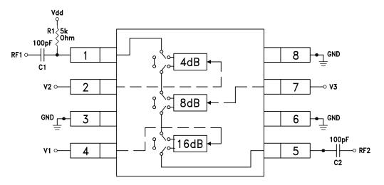
DC blocking capacitors C1 & C2 are required on RF1 & RF2. Choose  $C1 = C2 = 100 \sim 300 \text{ pF}$  to allow lowest customer specific frequency to pass with minimal loss. R1 = 5K Ohm is required to supply voltage to the circuit through either PIN 1 or PIN 5.
