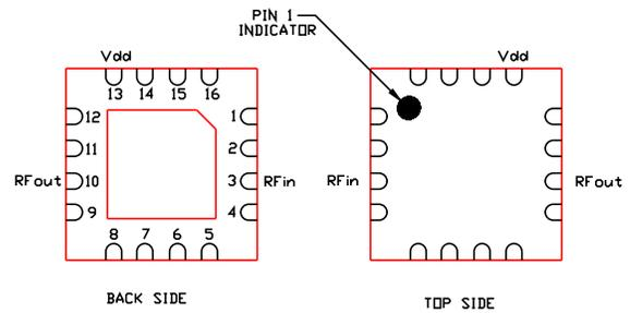
We recommend to ground all non-connected pins and to have as many via holes as possible under the ground paddle.
