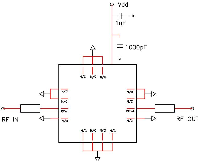
The input requires DC blocking capacitor if DC voltage is present on the input RF line.
