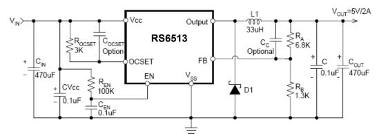
Note:  $V_{OUT} = V_{FB} x (1+R_A/R_B)$  $R_B=0.7K\sim5K \text{ ohm}$
