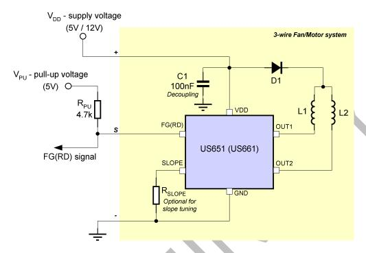
Typical computer fan application circuit
