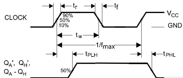
**Figure 1. Switching Waveform**
