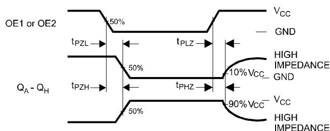
**Figure 3. Switching Waveform**
