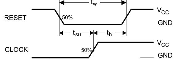
**Figure 2. Switching Waveform**
