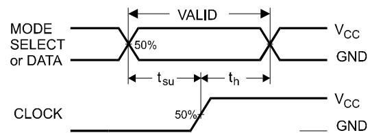
**Figure 4. Switching Waveform**
