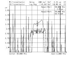
Horizontal: 0.6MHz/Div Vertical: 10dB/Div Horizontal: 0.6MHz/Div Vertical: 200ns/Div
